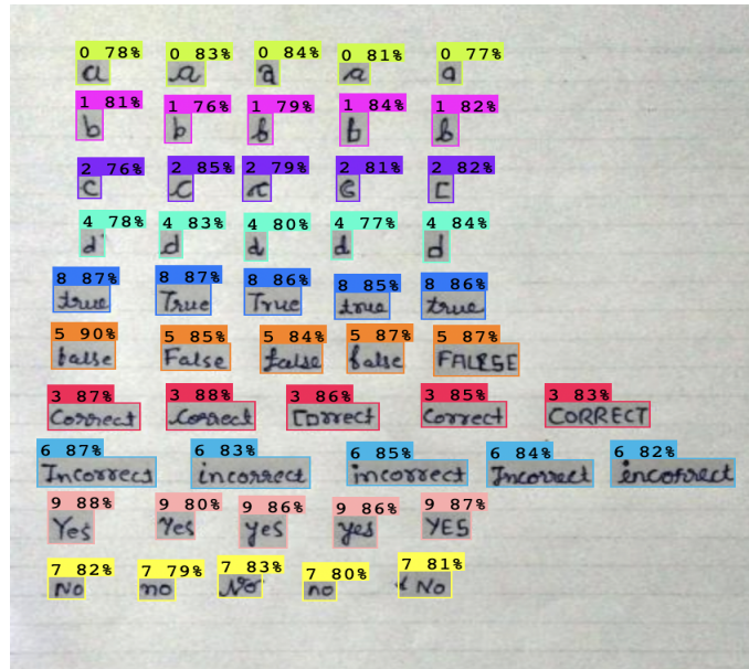
Figure 3.2: Result of YOLO Model with predicted class confidence on detected bounding box on ruled page
