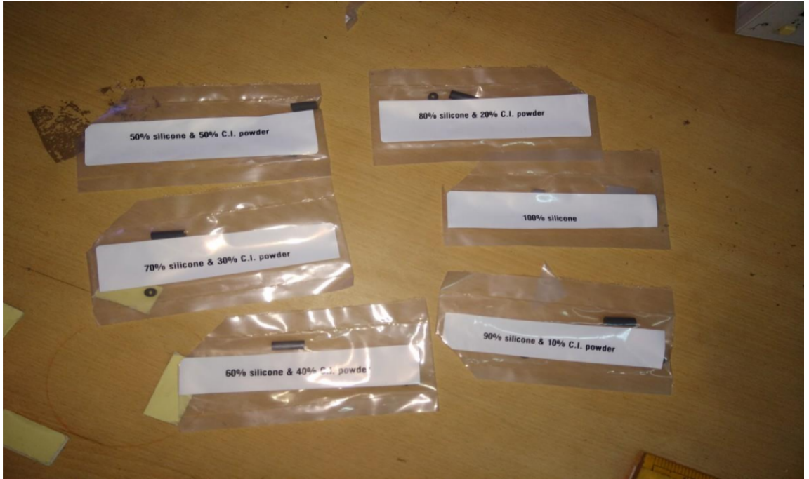
Figure 4.15: Toroidal-shaped CISR sleeves for coaxial air line
