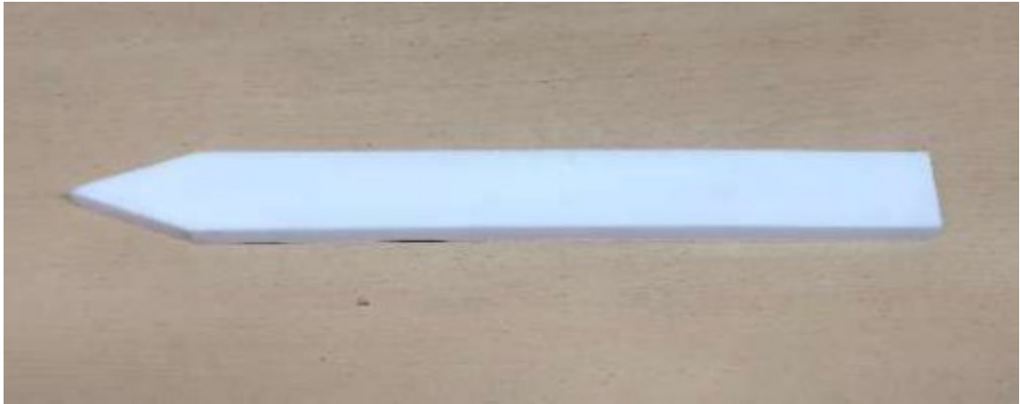
Figure 4.11: Photograph of tapered dielectric waveguide section for WR-137 frequency bands
