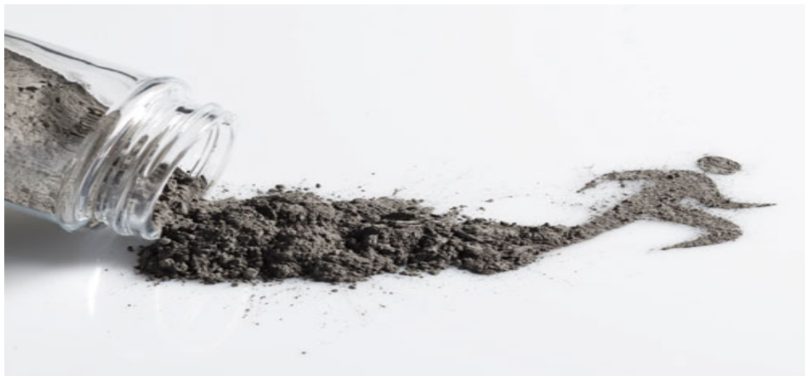
Figure 3.2: Carbonyl Iron Powder [19]
