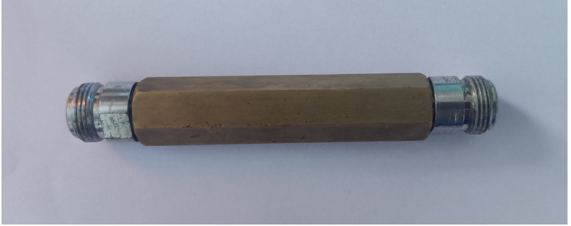
Figure 4.4: The photograph of coaxial air line fixture
