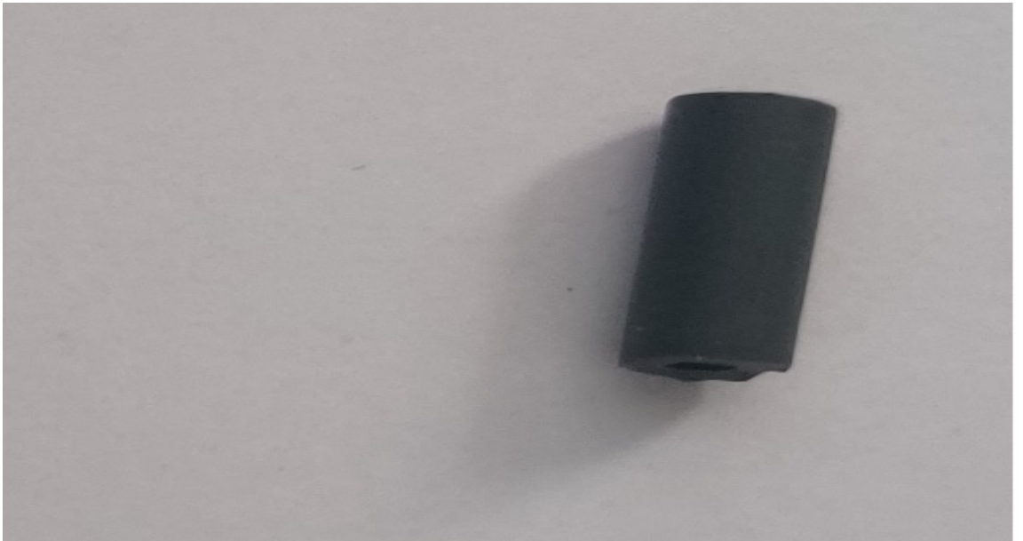
Figure 4.5: Photograph of toroidal shape sleeve CISR.
